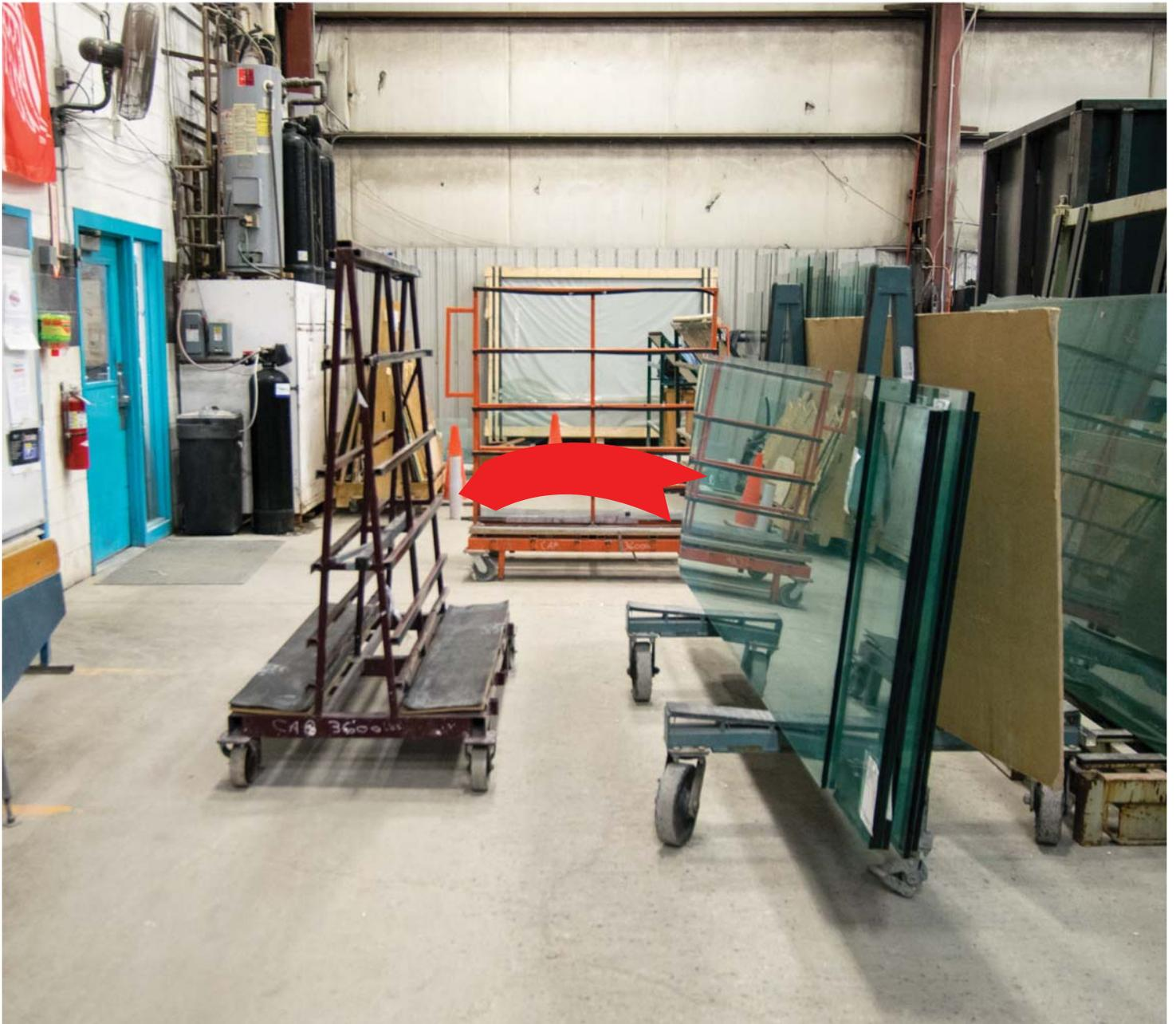
A cart used to stack glass on when trying to reach glass in the back of a stack
