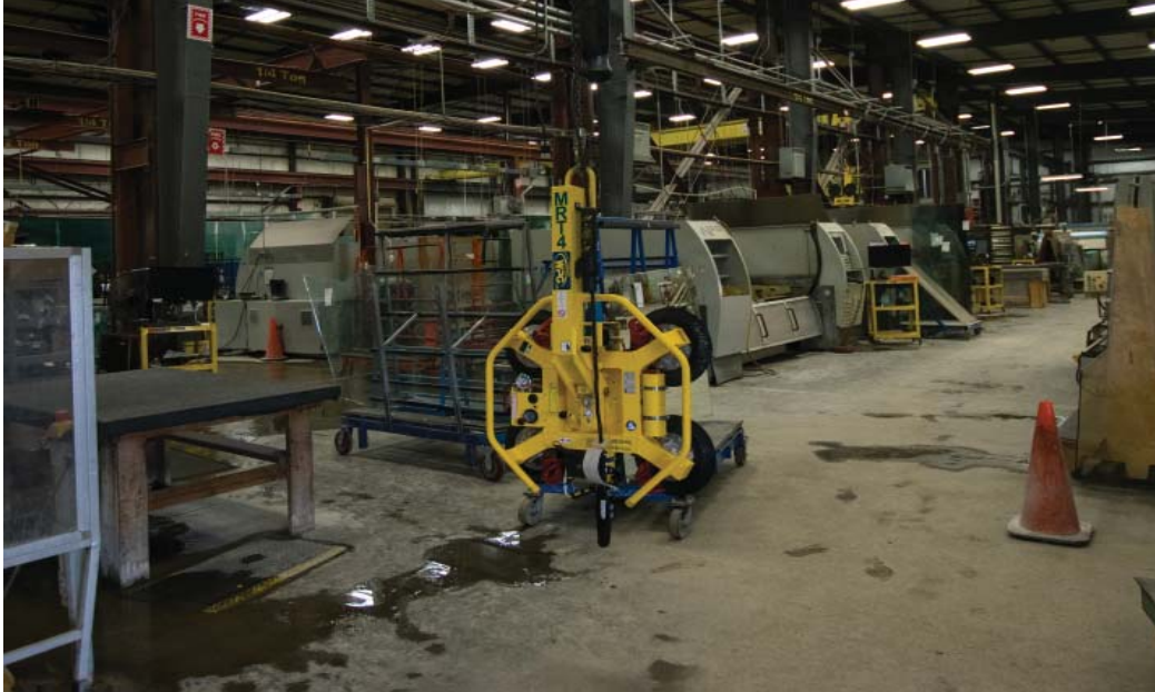
Suction cups for lifting glass
